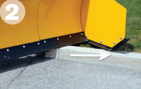
2 The side panel rides on top of the curb, while the rest of the plow remains flat.
