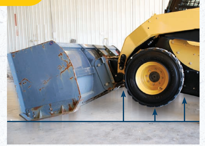
When other snow pushers are lowered, the front tires are lifted off the ground, reducing traction.
