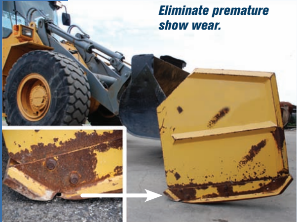
The Sectional Sno-Plow's shoes always automatically lay flat on the surface. Made of AR-400 hardened steel, the shoe will last several winters of commercial use.
