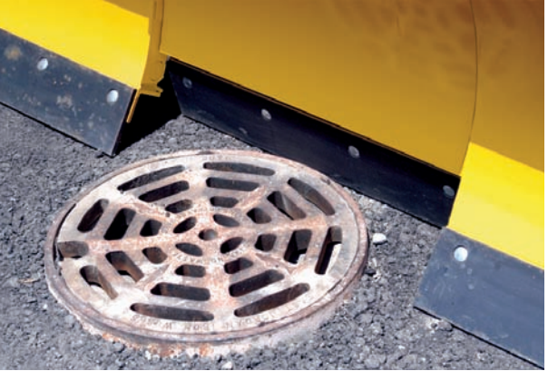
The spring trip steel cutting edge is forced backward upon impact and easily clears smaller obstacles.
