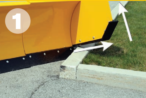
1 The side panel moves upward to clear obstacles such as curbs.
